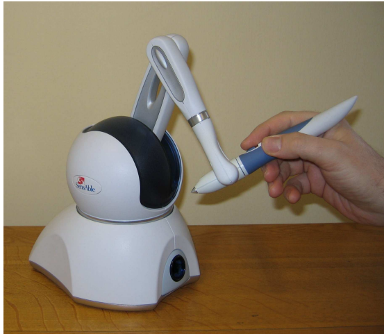
Figure 2. A picture of a SensAble Technologies' PHANTOM Omni Haptic Device ( www.sensable.com ) as used in SoundBar experiment. The user interacts with the "pen" which also contains two buttons for interaction.
