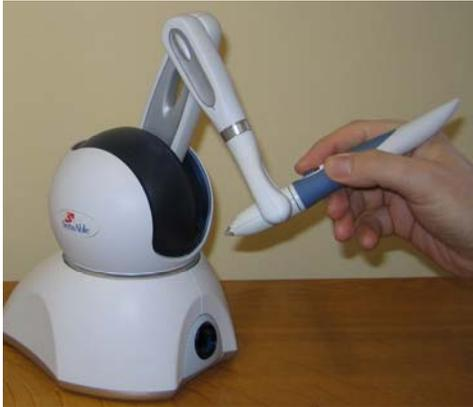
**figure 2.** The PHANTOM Omni haptic device used by participants to interact with the virtual graph. The user moves the “pen” like a 3D mouse. The device monitors this and uses motors to resist the user’s movement.
