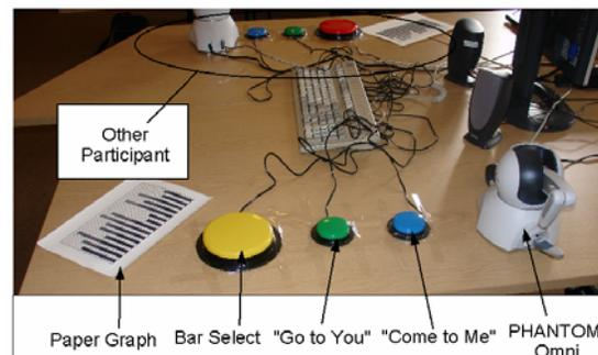
**figure 4.** The experimental setup for each participant.
